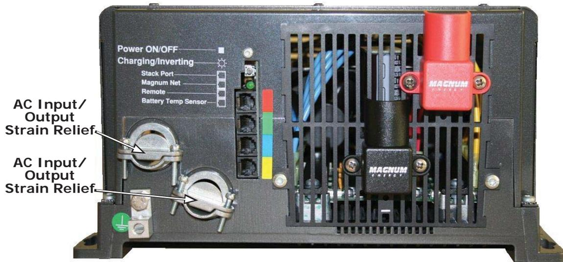
Figure 2-8, RD Series Inverter/Charger - AC Wiring
