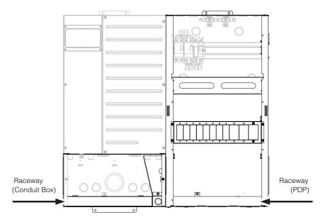
Figure 2-10 Example of raceways in a single-inverter system
