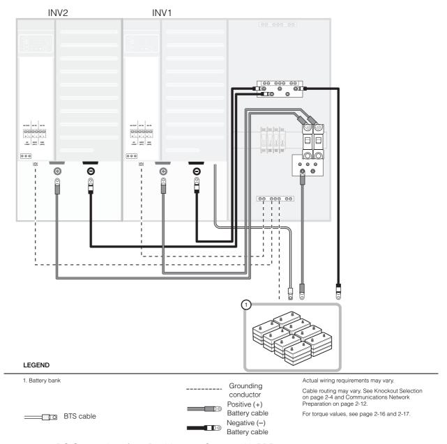
Figure 3-24 DC Connections for a Dual-Inverter System with PDP
