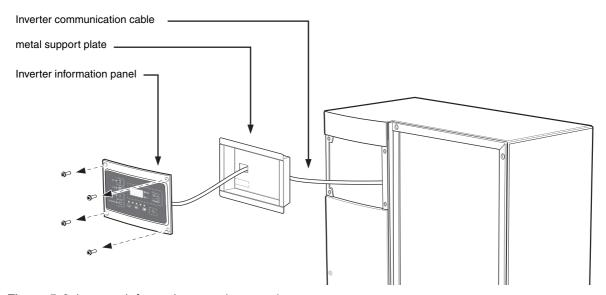
Figure 5-2 Inverter information panel removal
