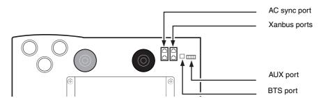
Figure 4-4 Conext XW+ Inverter/Charger communication ports
