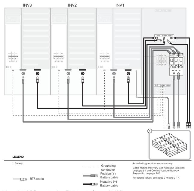
Figure 3-25 DC Connections for a Triple-Inverter System with PDP
