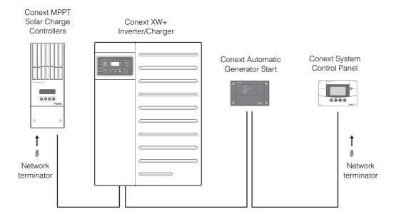
Figure 4-1 Xanbus Network System (Example)
