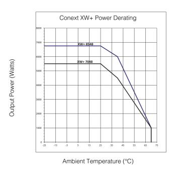
Figure A-2 Output Power Versus Ambient Temperature
