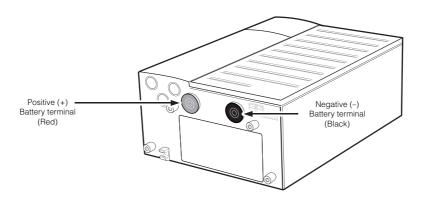
Figure 3-6 Battery terminals (bottom of Conext XW+)
