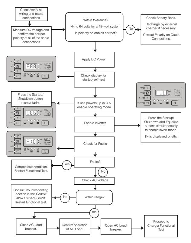
Figure 3-21 Functional Test for Single Inverter Systems
