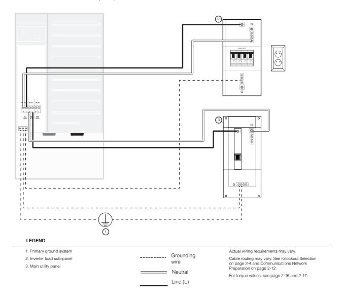
Figure 3-13 Wiring to the Inverter Load Sub-Panel or Utility Grid (no PDP)
