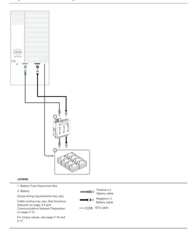
Figure 3-8 DC Connections to a Single Inverter without a PDP
