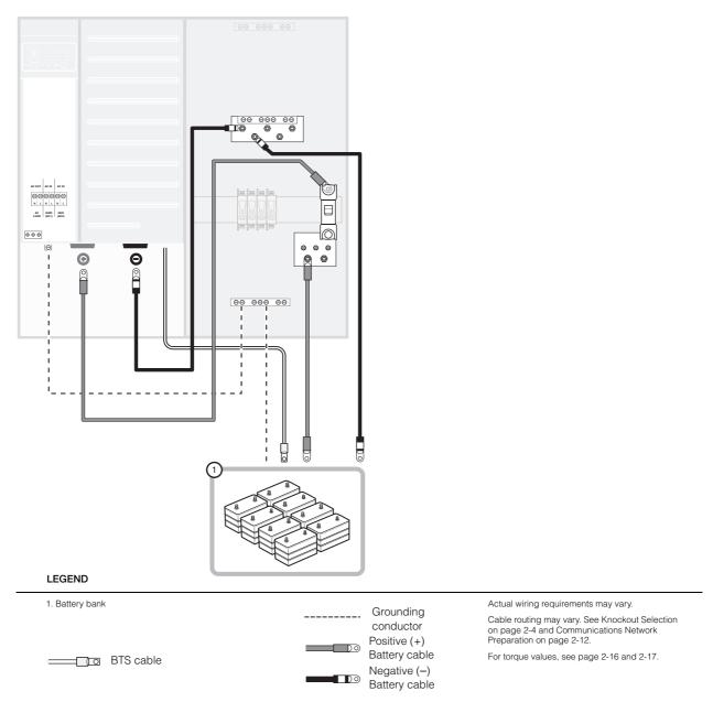
Figure 3-23 DC Connections for a Single-Inverter System with PDP
