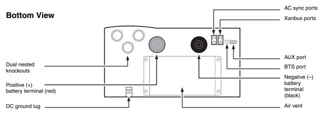
Figure 1-2 Conext XW+ Inverter/Charger Features
