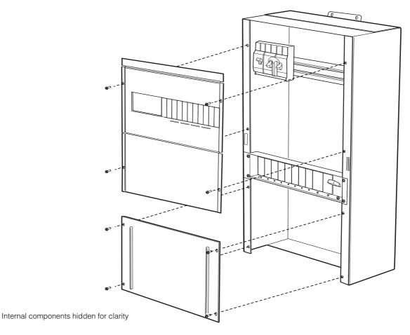
Figure 3-22 Conext XW+ Power Distribution Panel faceplate removal
