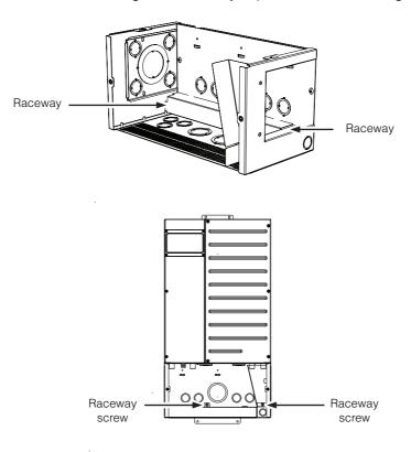
Figure 4-5 XW+ Conduit Box raceways
