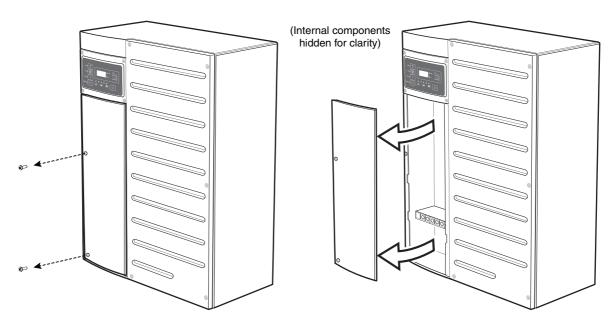
Figure 3-1 AC access panel removal
