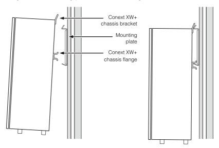
Figure 2-6 Wall-mounting the Conext XW+
