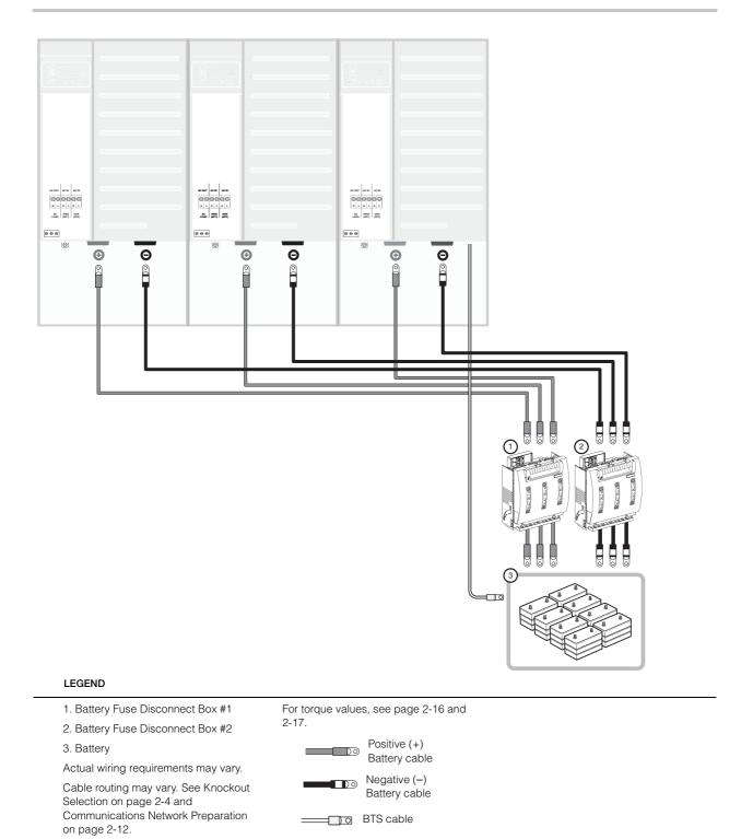
Figure 3-10 DC Connections for a Triple Inverter System without a PDP
