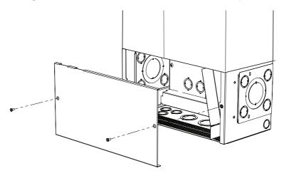
Figure 2-9 Conduit Box installation
