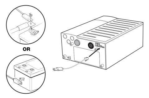
Figure 3-5 Battery Temperature Sensor Installation
