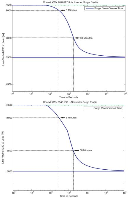
Figure A-1 Conext XW+ AC Overload Capability
