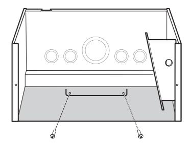
Figure 2-8 Wall-mounting the Conduit Box
