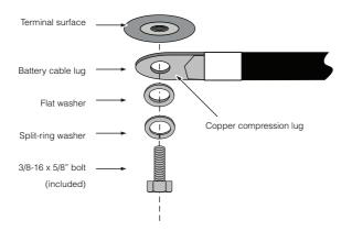
Figure 3-7 Battery cable connection
