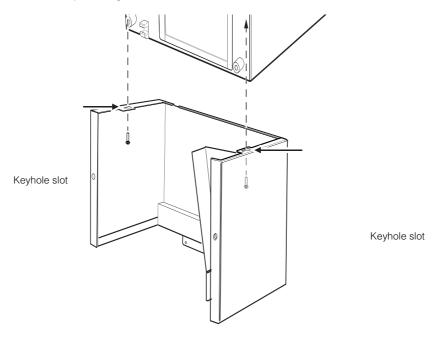
Figure 2-7 Conduit Box keyhole alignment
