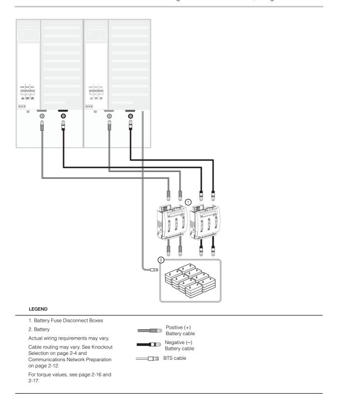
Figure 3-9 DC Connections for a Dual Inverter System without a PDP
