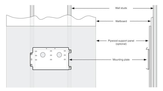
Figure 2-4 Mounting plate centered on wall studs
