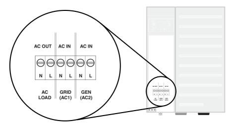
Figure 3-11 AC terminal block
