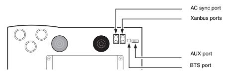
Figure 3-2 Conext XW+ Inverter/Charger communication ports
